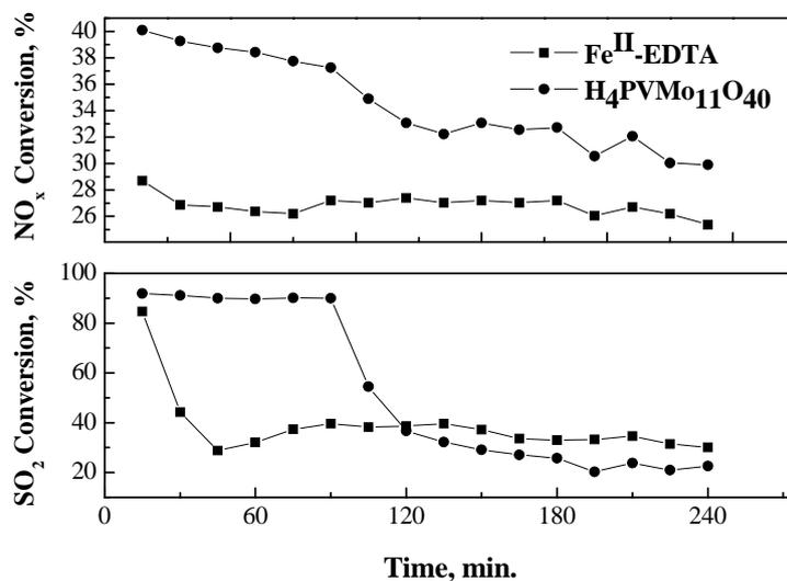
Figure 2. Comparison of the new absorbent with Fe<sup>II</sup>-EDTA
