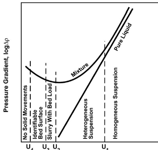
Figure 1. Pressure Drop Variation versus Velocity
