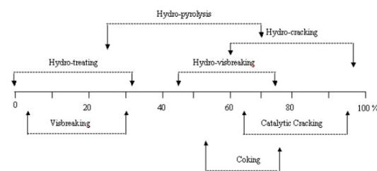
Fig. 14 Extent of feedstock conversion in various processes [18, 6]
