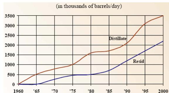
Fig.10 The trend of global heavy oil hydro-processing [17]
