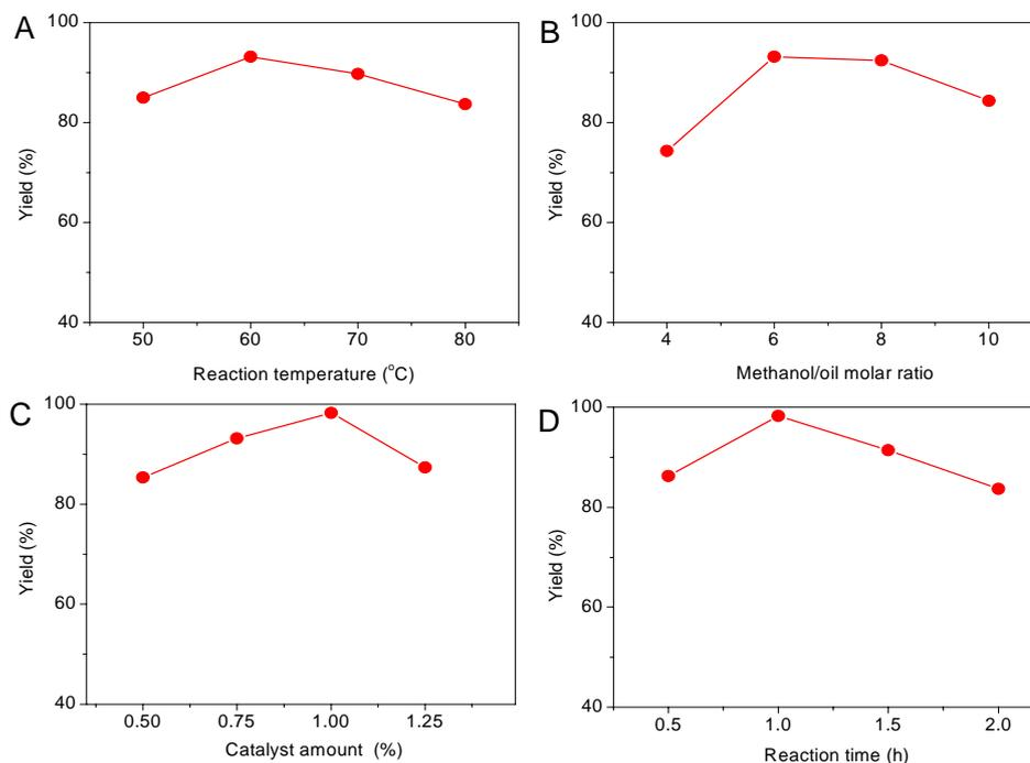
Fig 2. Effects of variables on biodiesel yield: (a) reaction temperature (b) methanol/oil molar ratio (c) catalyst amount (d) reaction time.
