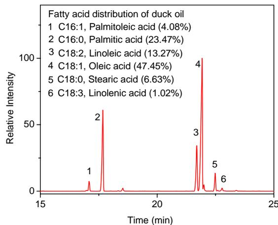
Fig 1. The GC-MS graph of roast duck oil after methyl esterification
