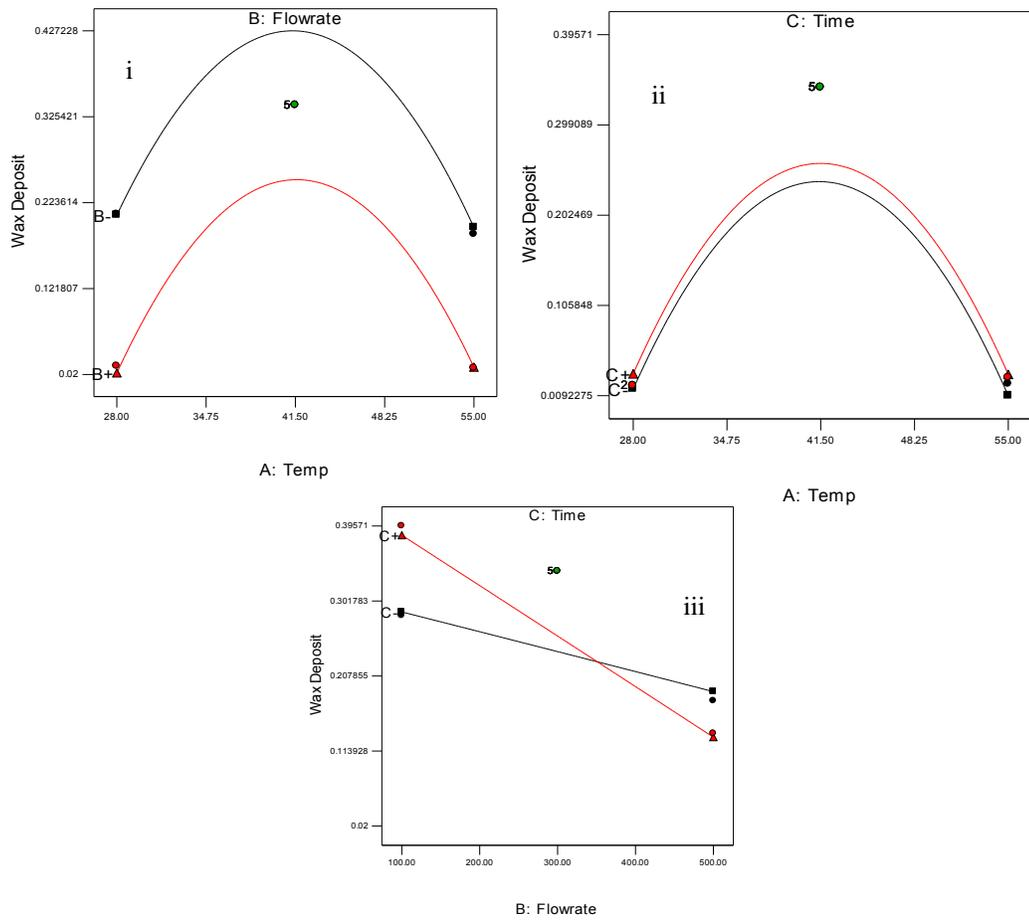
Figure 2 Two Factor interactions of variables on wax deposited
