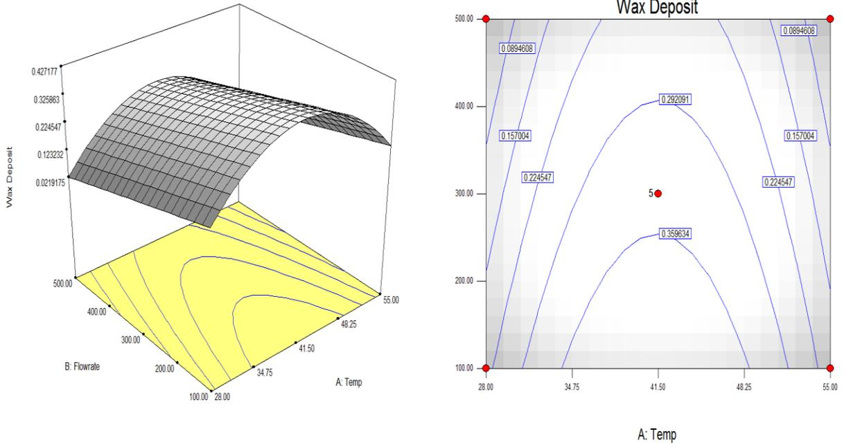
Figure 4 Surface plot of interaction between time and temperature on wax deposited.
