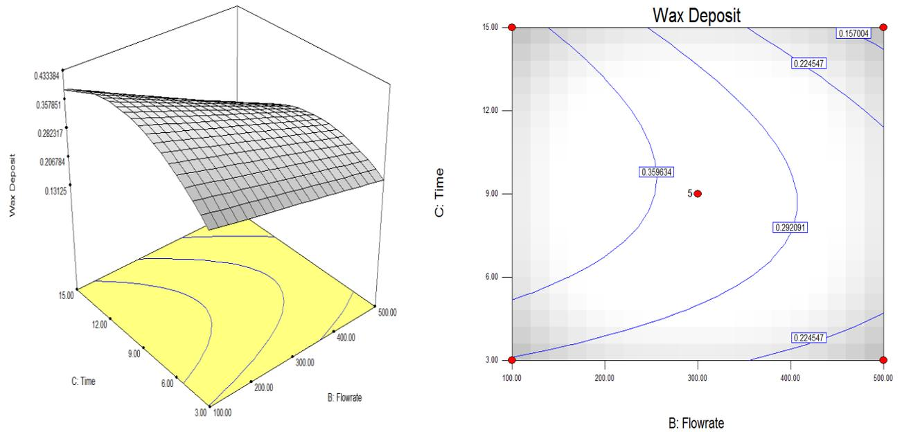
Figure 5 Surface plot of interaction between time and flowrate on wax deposited.
