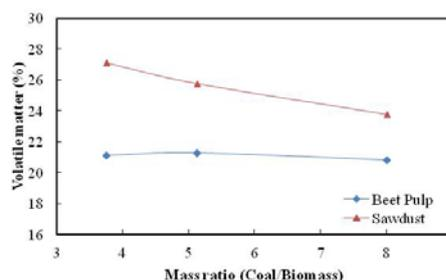
Fig.2. Effect of natural binders on the amount of volatile materials
