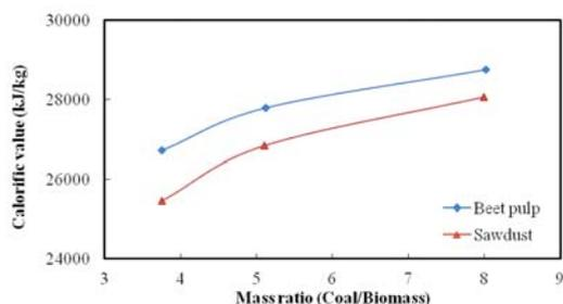
Fig.3. Effect of natural binders on the calorific value
