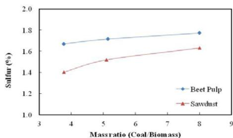
Fig.1. Effect of natural binders on the amount of sulfur
