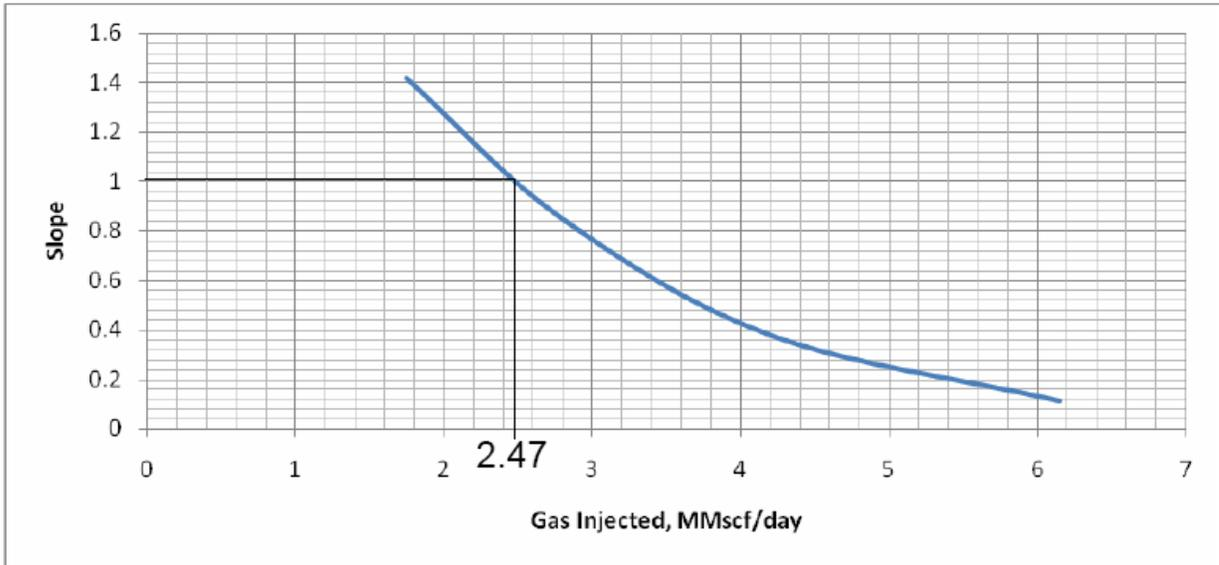
Fig. 3.3 Gas Injected at the Slope of 1
