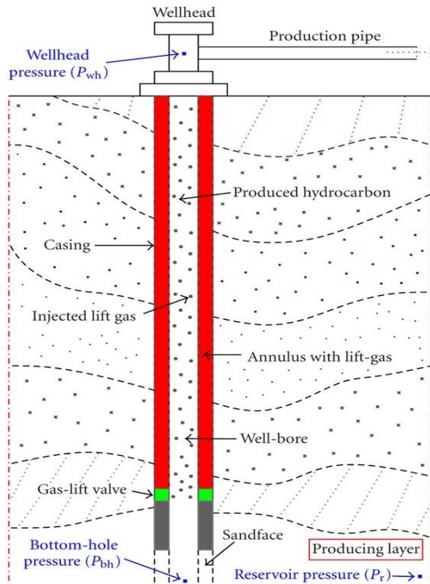
Fig 1.1 Gas Lift Well Schematic (Source: Brown, 1982)
