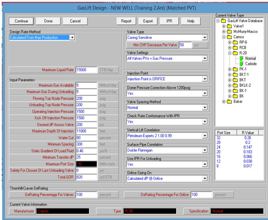
Fig. 2.2 PROSPER Interface for Gas Lift Design – New Well (Source: Petroleum Experts Limited)
