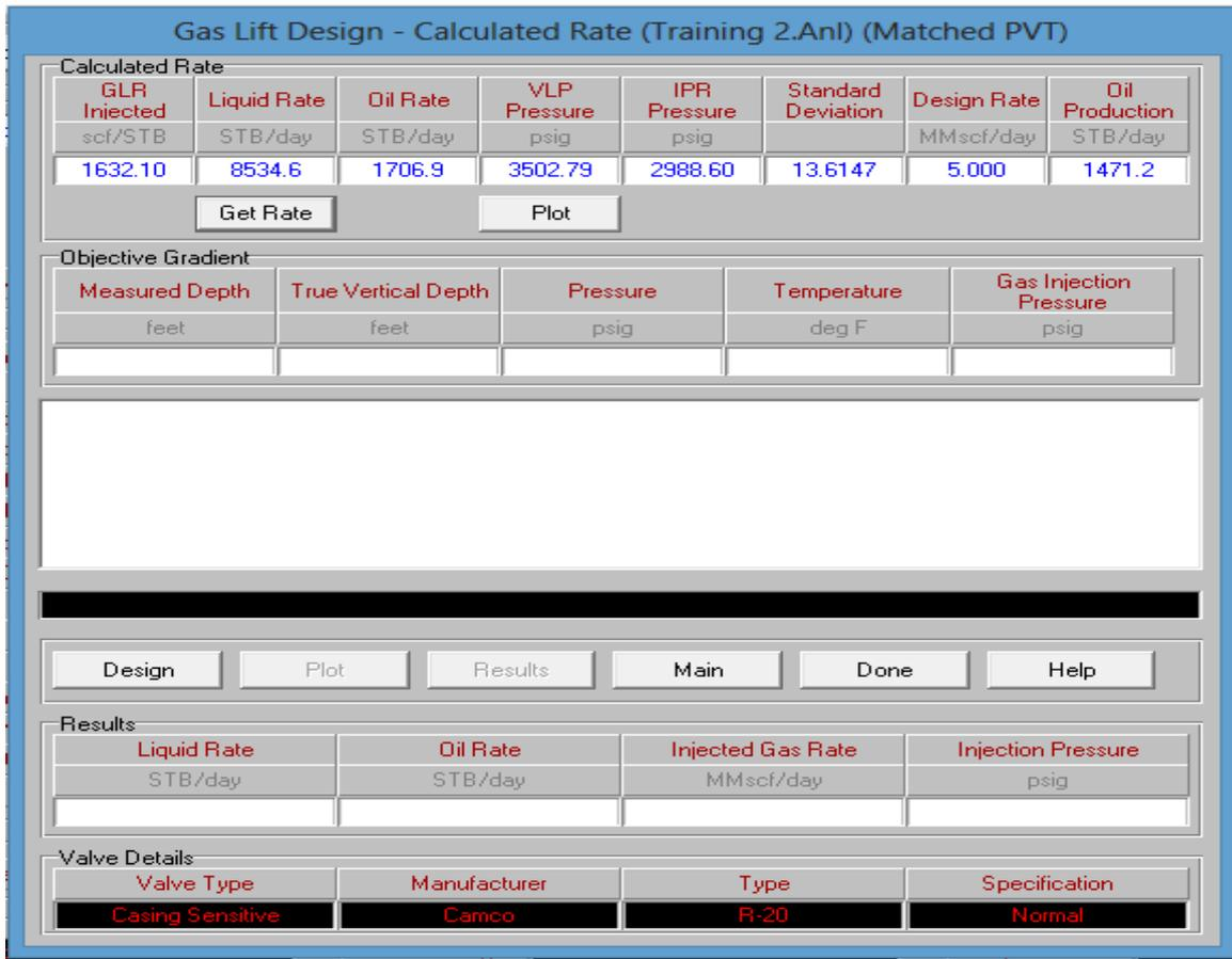
Fig. 2.4 PROSPER Interface for Gas Lift Design – Calculated Rate, with the Calculated Values (Source: Petroleum Experts Limited)
