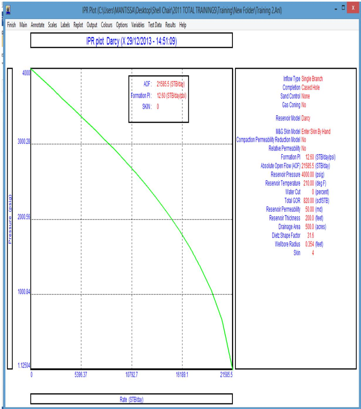
Fig. 2.8 PROSPER Interface – IPR Curve (Source: Petroleum Experts Limited)
