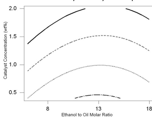
Fig. 3. Contour plots of ester yield vs. ethanol to oil molar ratio and catalyst concentration for the second-order model with reaction temperature of 57.5°C
