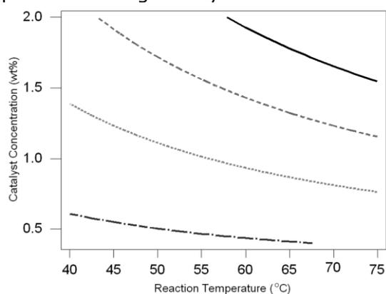
Fig. 2. Contour plots of ester yield vs. reaction temperature and catalyst concentration for the second-order model with ethanol to oil molar ratio of 12:1
