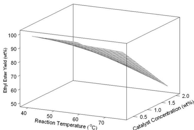
Figure 1. Response surface of ester yield vs. reaction temperature and catalyst concentration for the second-order model with ethanol to oil molar ratio of 12:1
