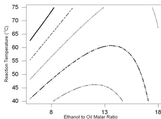
Fig. 4. Contour plots of ester yield vs. ethanol to oil molar ratio and reaction temperature for the second-order model with catalyst concentration of 1.2%
