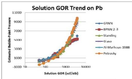
Figure 7 Solution Gas-Oil Ratio Trend on Bubble Point Pressure
