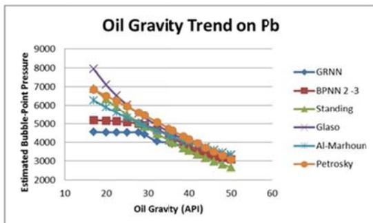
Figure 8 Oil Gravity Trend on Bubble Point Pressure
