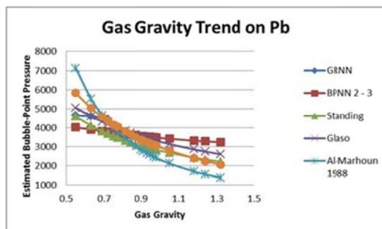
Figure 9 Gas Gravity Trend on Bubble Point Pressure
