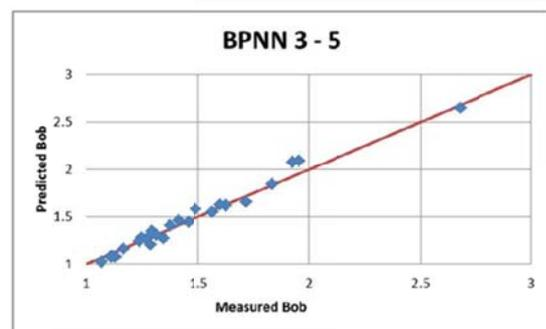
Figure 21 Cross Plot of BPNN model for  $B_{ob}$
