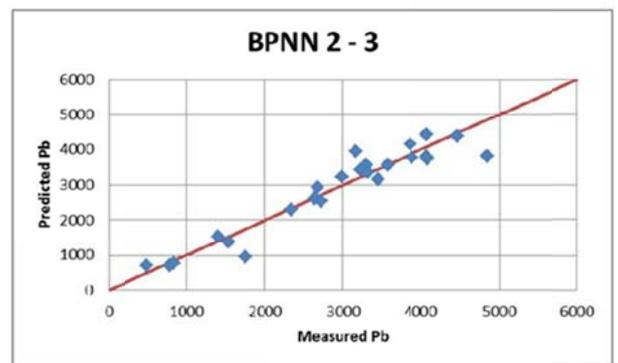
Figure 15 Cross Plot of BPNN model for  $P_b$
