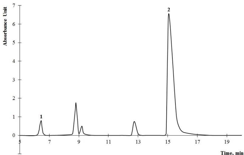
Figure 2. HPLC chromatogram of recrystallized lactide: 1 – lactic acid; 2 – D,L-lactide
