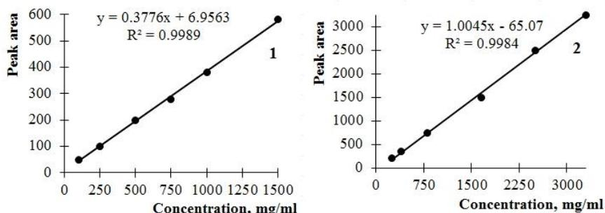
Figure 1. Calibration curves of the peak area versus concentration: 1 – lactic acid; 2 – D,L-lactide
