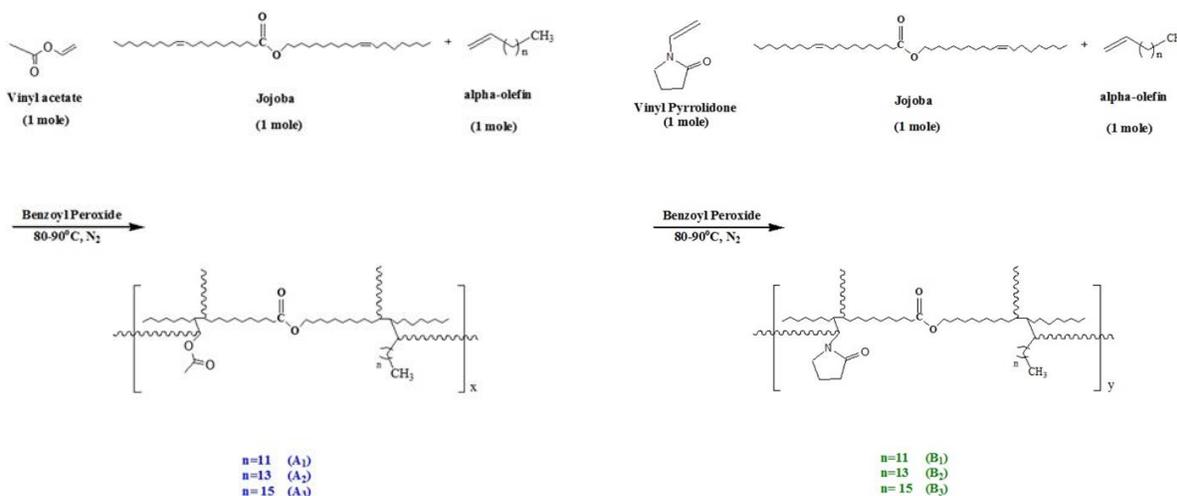
Scheme 1. (Jojoba: vinyl acetate:  $\alpha$ -olefins) terpolymers      Scheme 2. (Jojoba: vinyl pyrrolidone:  $\alpha$ -olefins) terpolymers
