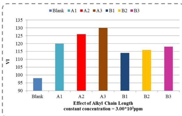
Fig. 1. Effect of alkyl chain length of  $\alpha$ -olefin used on VI of lube oil SAE-30 free of Additives
