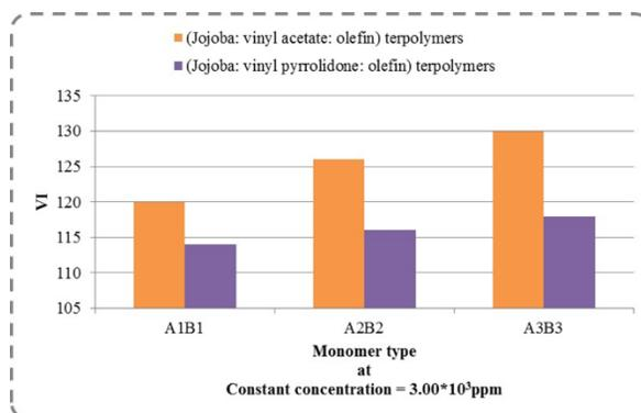
Fig. 2. Effect of Monomer Type on VI of lube oil SAE-30 free of Additives.
