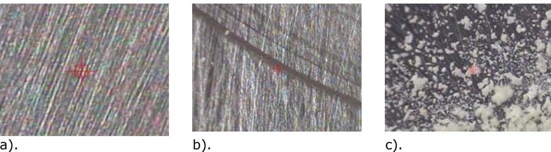
Fig. 4. Surface of the steel disk with roughness 0.08  $\mu\text{m}$  before (a) and after experiment: the track of friction with polymer roads (b) and with polymer particles (c) under load of 18 N, the linear velocity of 0.50 m/s
