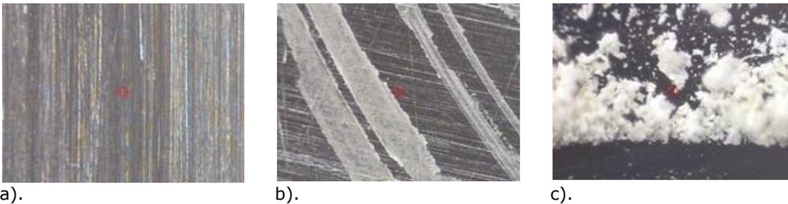
Fig. 2. Surface of the steel disk with roughness 0.15  $\mu\text{m}$  before (a) and after experiment: the track of friction with polymer roads (b) and with polymer particles (c) under load of 18 N, the linear velocity of 0.50 m/s
