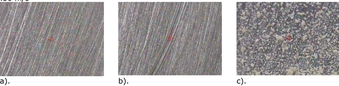
Fig. 3. Surface of the steel disk with roughness 0.08  $\mu\text{m}$  before (a) and after experiment: the track of friction with polymer roads (b) and with polymer particles (c) under load of 10 N, the linear velocity of 0.50 m/s
