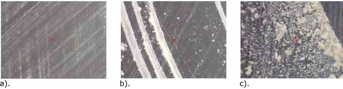
Fig. 1. Surface of the steel disk with roughness 0.15  $\mu\text{m}$  before (a) and after experiment: the track of friction with polymer roads (b) and with polymer particles (c) under load of 10 N, the linear velocity of 0.50 m/s
