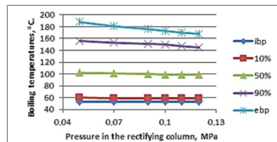
Fig. 5. Boiling temperatures (D86) vs pressure in the rectifying column.
