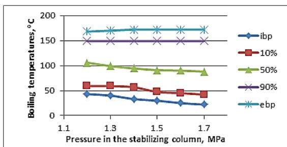
Fig. 4. Boiling temperatures (D86) vs pressure in the stabilizing column.
