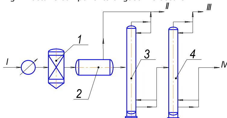
Fig. 1. PFD of gasoline conversion on zeolite catalysts: 1 – reactor; 2 – separator; 3 – stabilizing column; 4 – rectifying column; flows: I – feedstock; II – hydrocarbon gases; III – gasoline; IV – heavy residue.
