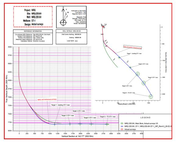
Figure 6. Actual horizontal well trajectory- the planned versus the reality <sup>[10]</sup>
