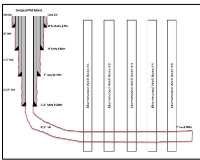
Figure 5. Conceptual Well Scheme for an ERD Project
