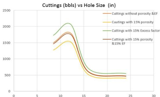
Figure 3. Amount cuttings generated in M-16 ERD well
