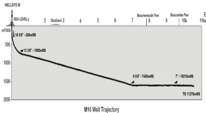
Figure 1. Actual Trajectory of 11-km ERD Well at Wytch Farm [18]
