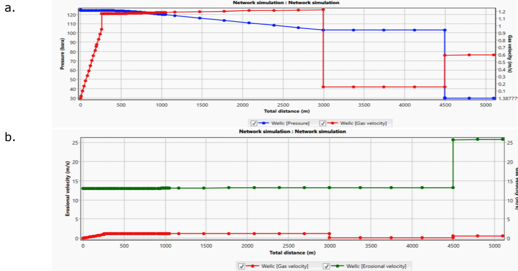
Figure 6. Gas parameters variation of well C with 12.7 nozzle size: a. Gas speed and pressure distribution; b. Gas velocity and erosion velocity distribution- Case 2
