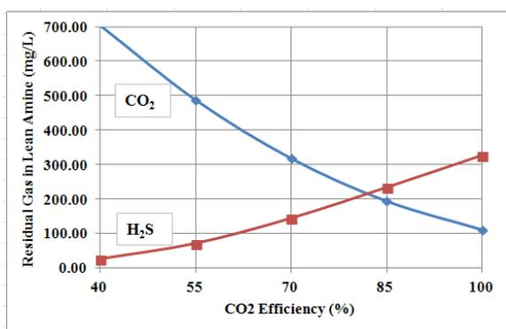
Figure 2. The changes of residual H<sub>2</sub>S and CO<sub>2</sub> in the lean amine vs. CO<sub>2</sub> efficiency
