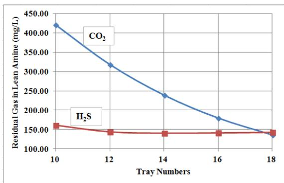
Figure 3. The changes of residual H<sub>2</sub>S and CO<sub>2</sub> in the lean amine vs. tray numbers
