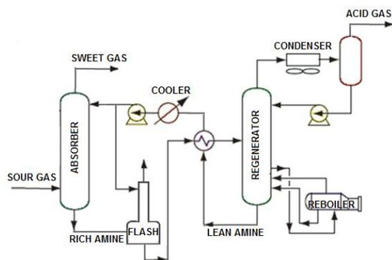
Figure 1. Schematic diagram of a typical amine sweetening unit
