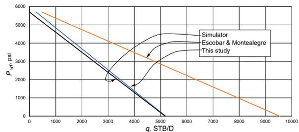
Figure 7. IPR curve,  $q$  vs  $P_{wf}$ , obtained by simulation versus flow calculated with different correlations excluding Joshi's correlation
