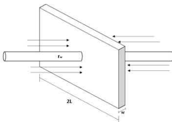
Figure 1. Diagram of fluid flow from the reservoir to the fracture
