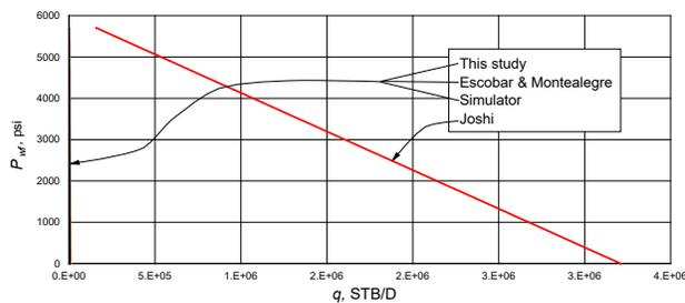
Figure 6. IPR Curve,  $q$  vs  $P_{wf}$ , obtained by simulation versus flow calculated with different correlations of the literature and the one from this study
