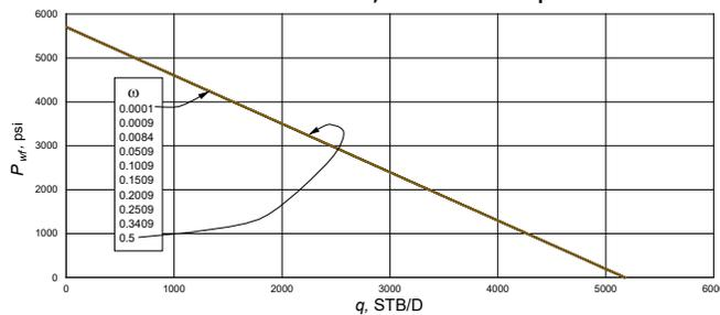
Figure 2. Simulated IPR curve,  $q$  vs  $P_{wf}$ , using different values of  $\omega$  and a fixed value of  $\lambda$  and equal to  $1 \times 10^{-6}$
