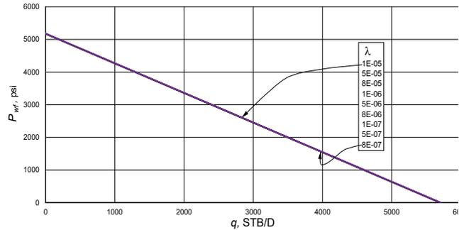
Figure 4. Simulated IPR curve,  $q$  vs  $P_{wf}$ , using different values of  $\lambda$  and a fixed  $\omega$  value of 0.0084
