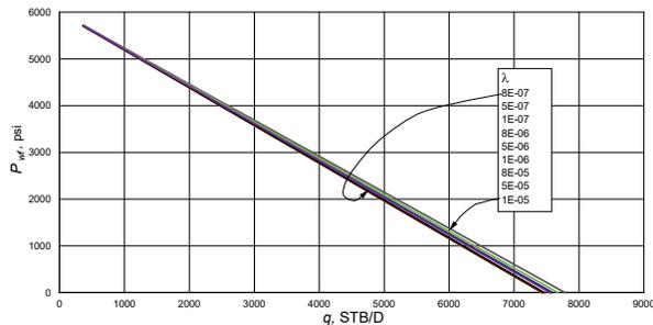
Figure 5. Simulated IPR curve  $q$  vs  $P_{wf}$ , with the new correlation, Eq. 7, using different values of  $\lambda$  and a fixed  $\omega$  value of 0.0084
