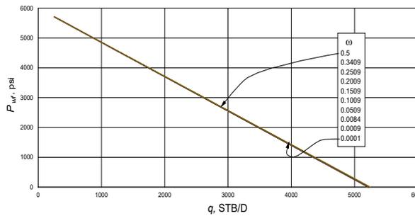
Figure 3. IPR curve,  $q$  vs  $P_{wf}$ , from the correlation of this study using different values of  $\omega$  and a set  $\lambda$  value of  $1 \times 10^{-6}$
