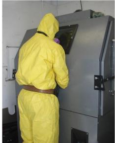
Figure 6. Isolated cabinet for NORM decontamination.
