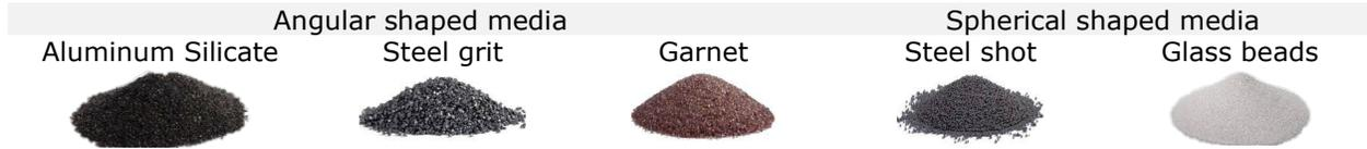
Figure 2 Examples of Different blasting materials.
