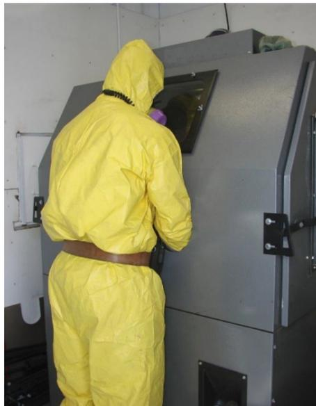
Figure 6. Isolated cabinet for NORM decontamination.
