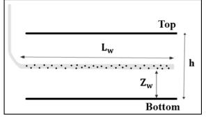
Figure 1.Schematic representation of a horizontal production well <sup>[3]</sup> As shown in Figure 1, a well with the horizontal length of  $L_w$  is drilled in a reservoir with thickness *h* in a way that the distance from the lower horizontal line of the reservoir is  $Z_w$ .
