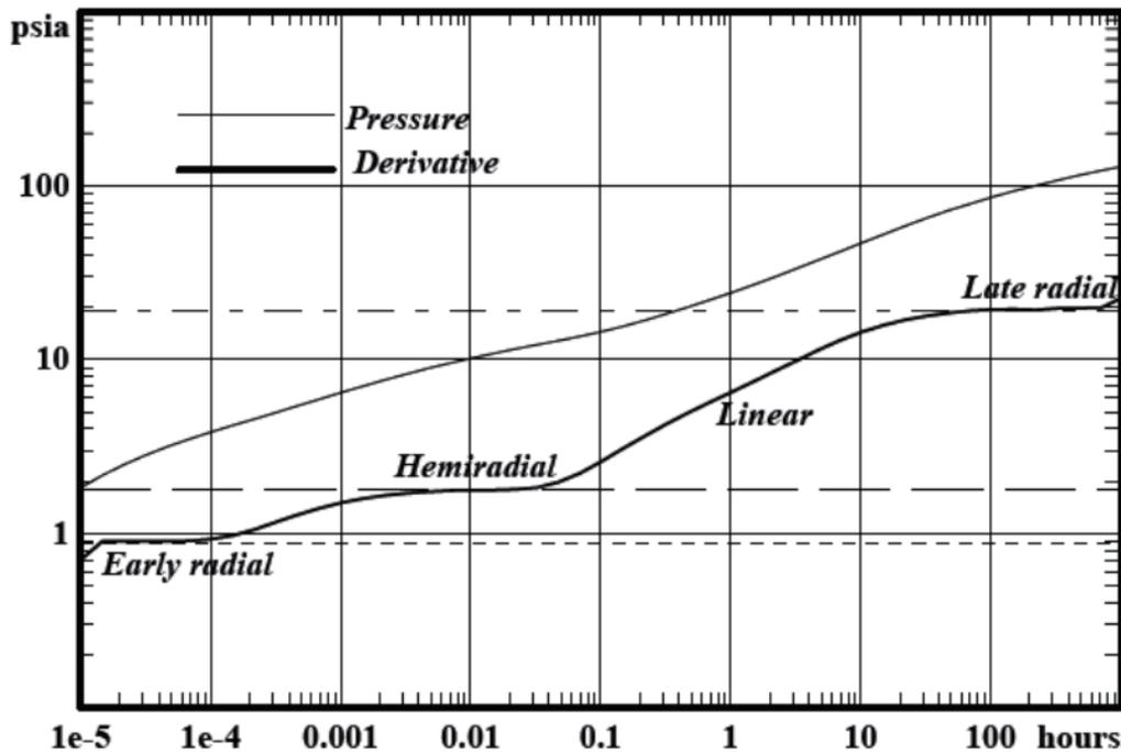
Figure 6. Pressure and pressure derivative curves in a horizontal well [4]
