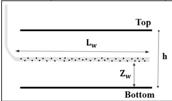
Figure 1. Schematic representation of a horizontal production well [3]
