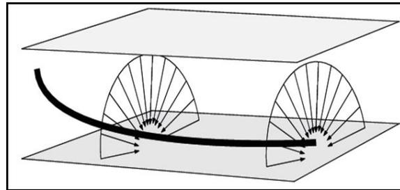
Figure 3. Semi-radial flow [4]
