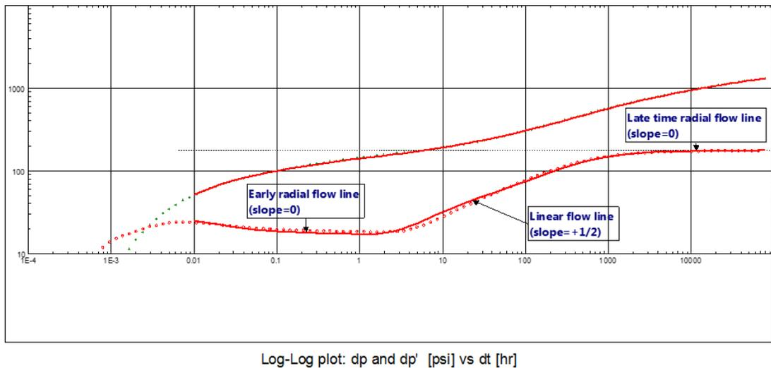
Figure 8. Pressure and pressure derivative diagram of the horizontal well after performing matching procedure
