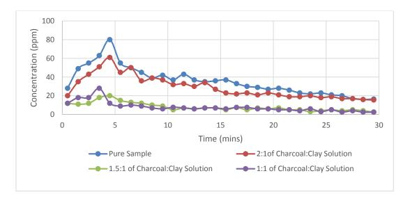
Figure 3.1. The temporal variation of CO emission levels from the pure and the formulated charcoal samples
