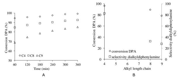
Figure 3. The conversion of alkenes C4, C8 and C9 using Fulcat 22B at 160°C (A), the conversion of the particular alkenes at the  $180^{th}$  minute of the alkylation process, and the total selectivity of dialkyldiphenylamine using Fulcat 22 B (B)
