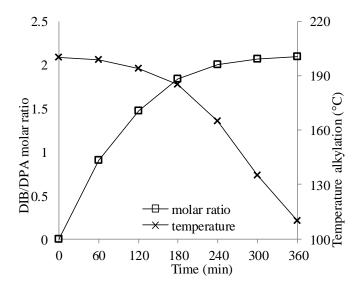
Figure 7. The temperature profile for the optimum conversion of DPA and the selectivity of (DODPA) and the dosing time f the DIB
