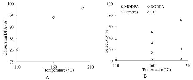
Figure 2. The effect of reaction temperature on the conversion of DPA (A) and the overall selectivity of isomers (B) using Fulcat 22B after 300 minutes of alkylation
