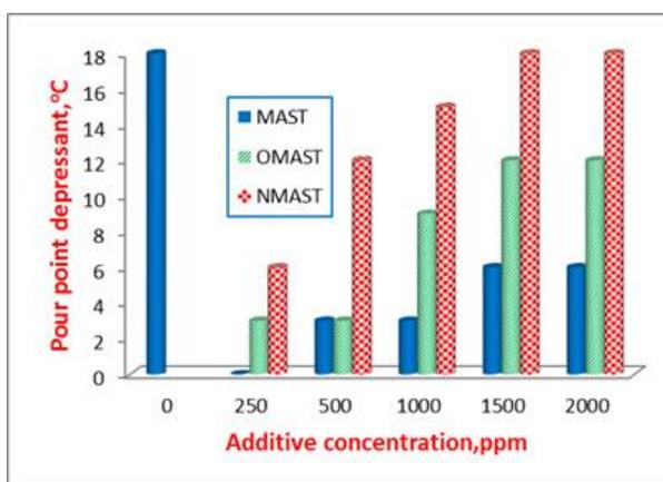
Figure1. Influence of additive on the pour point of gas oil
