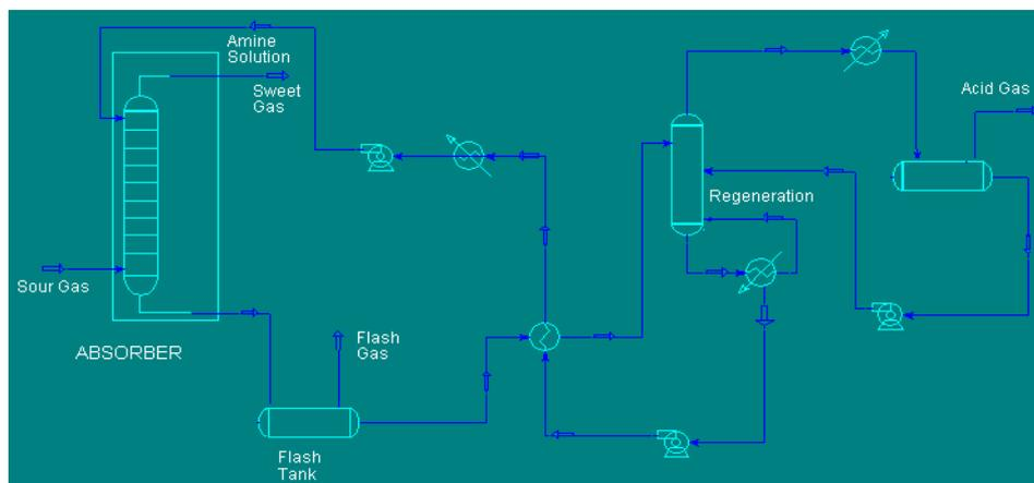
Fig (1): Process Flow Diagram of amine-sweetening unit
