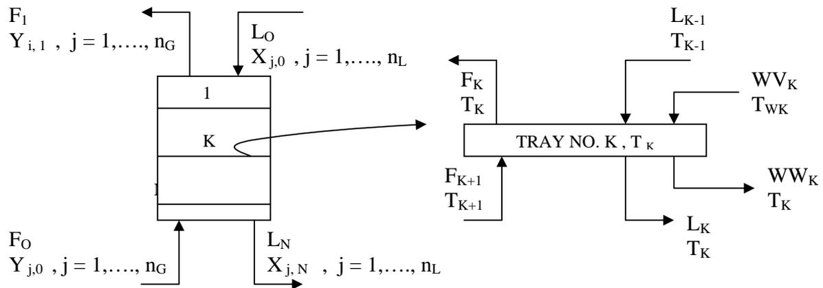
**Fig (2): Schematic of Absorber Tower**
