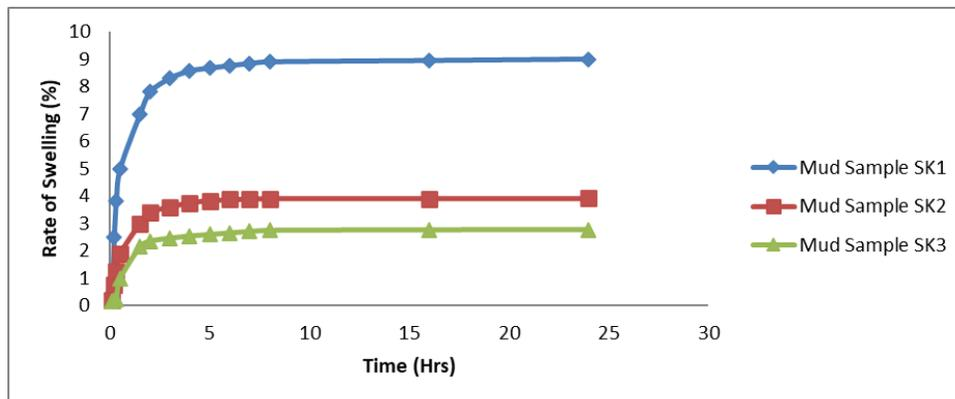
Figure 3. Rate of swelling rate vs time for various DMs
