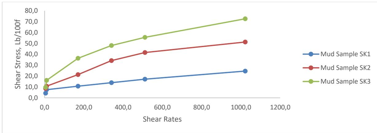
Figure 1. Shear stress and shear rate for mud samples SK1, SK2 and SK3
