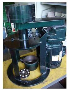
Figure 1. Hardgrove grindability index machine [19]
