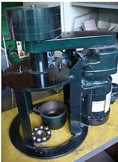
Figure 1. Hardgrove grindability index machine [19]
