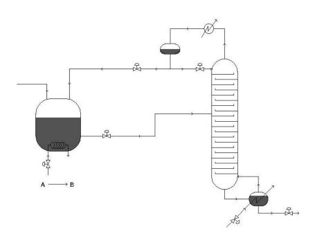
Figure 1- Process including one reactor and one distillation column.
