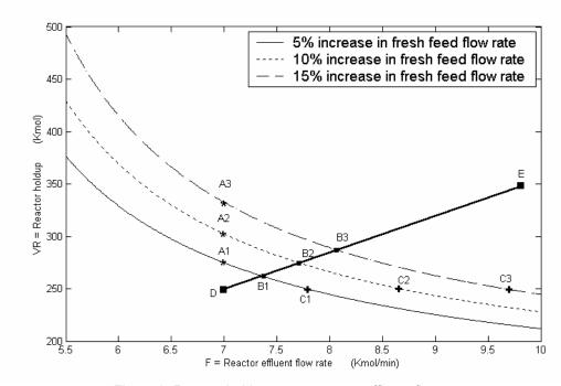
Figure 2- Reactor holdup versus reactor effluent flow rate.
