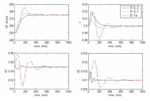
Figure 7- Variations of system states versus time for the structures B\_1a, first and second proposed structures due to 10% increases in feed flow rate.
