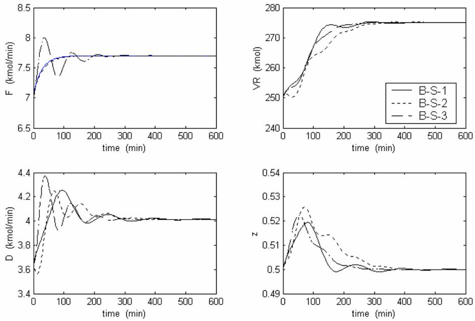
Figure 3- Variations of system states versus time for the three control structures with two concentration loops due to 10% increase in feed flow rate.
