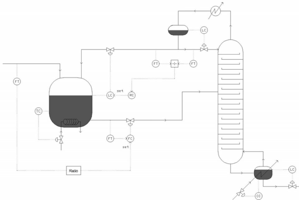
Figure 5- First proposed control structure.
