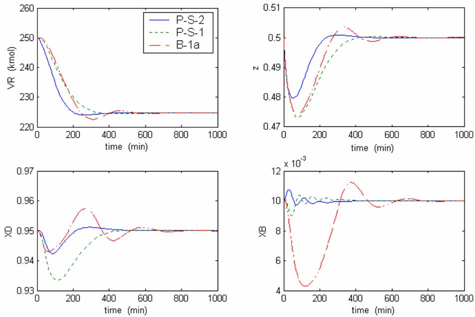
Figure 8- Variations of system states versus time for the structures B\_1a, first and second proposed structures due to 10% decreases in feed flow rate.
