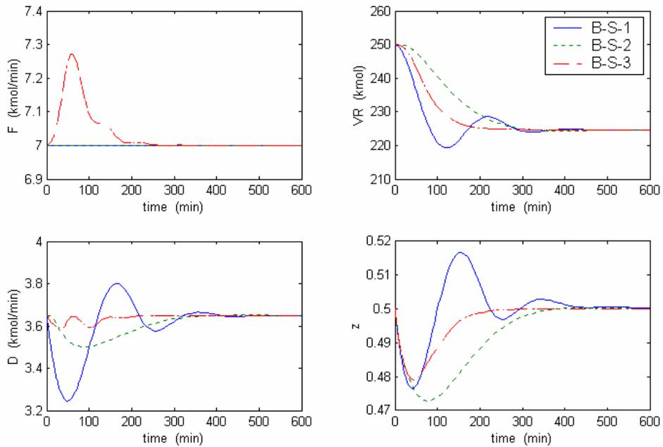
Figure 4- Variations of system states versus time for the three control structures with two concentration loops due to 10% decrease in feed flow rate.
