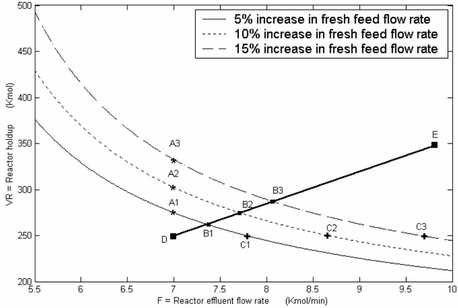
Figure 2- Reactor holdup versus reactor effluent flow rate.
