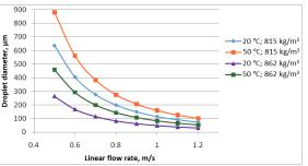
Fig. 3. Dependence of the droplet diameter on the linear flow rate, temperature, and oil density
