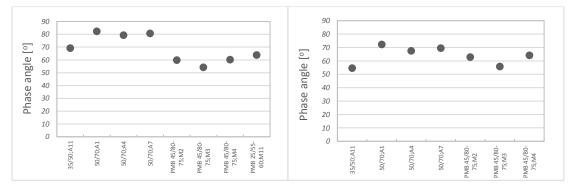
Figure 5. Values of phase angle from the DSR test at 50°C (left) and 25°C (right)
