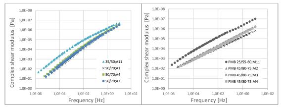
Figure 3. Complex modulus of non-modified (left) and modified (right) bitumen samples at 25°C reference temperature
