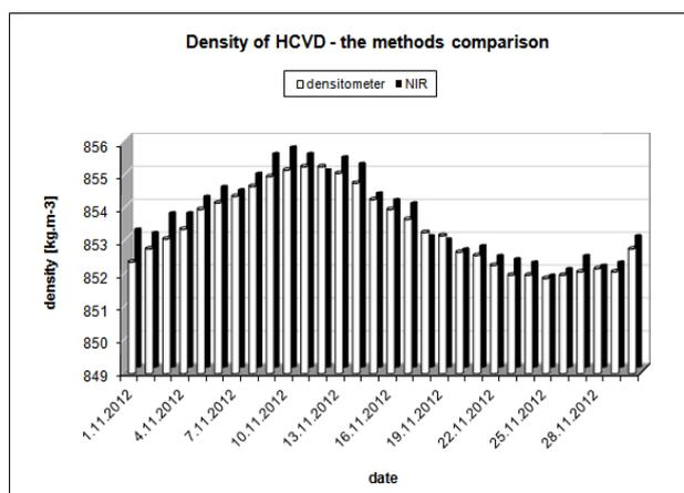
Fig. 3 Comparison of measured values of HCVD density by NIR spectrometry and instrumental densitometry.
