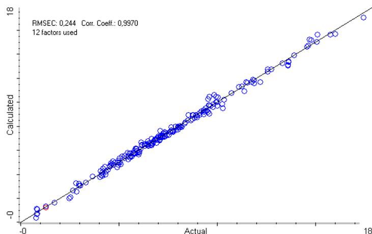
Figure 1 NIR model for determination of aromatic hydrocarbons in straight-run gasoline.
