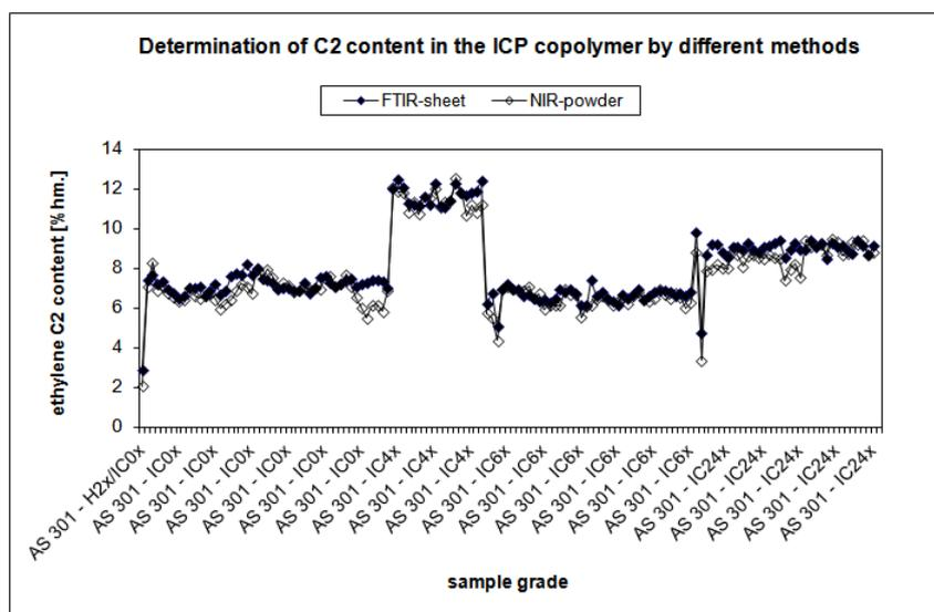
Figure 6: Comparison of results for the determination of ethylene in co-polymers by the method NIR and FTIR.
