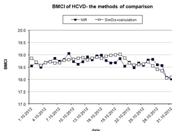
Fig. 4 Comparison of measured values BMCI by NIR spectrometry and SIMDIS.
