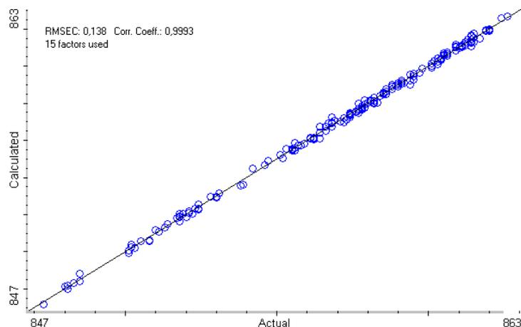
Figure 2 NIR model for density determination of hydrocracking vacuum distillates (HCVD).
