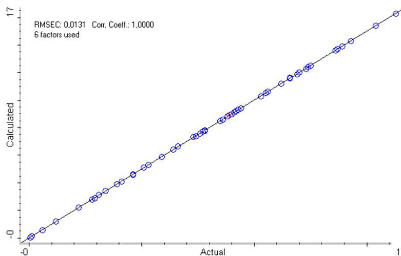
Figure 5 NIR model for the determination ethylene in propylene.
