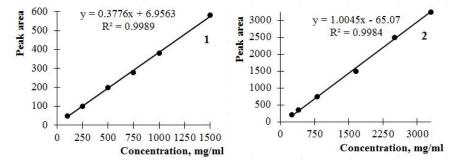
Figure 1. Calibration curves of the peak area versus concentration: 1 – lactic acid; 2 – D,L-lactide
