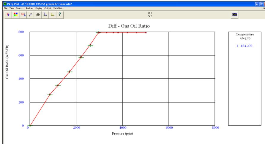
Figure. 14. Differential liberation test – GOR match (RFR01 Oil sample)
