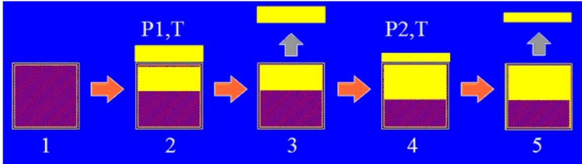
Figure. 1 A schematic illustration of the constant-volume depletion test
