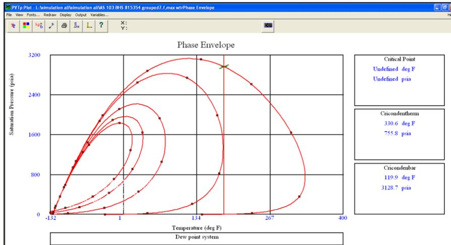
Figure. 6. Phase envelope match (RFR01Reconstructed sample)
