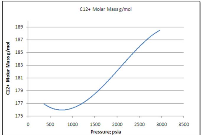
Figure. 3 Extending C12+ Molar Mass from CVD to the initial pressure
