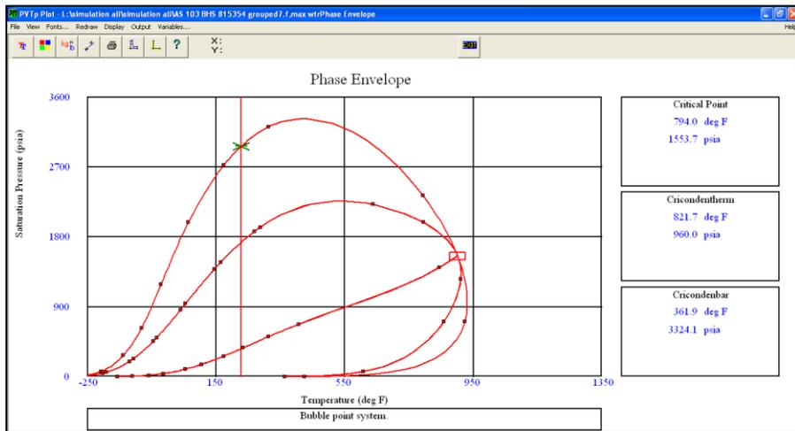
Figure. 10. Phase envelope match (RFR01 Oil sample)
