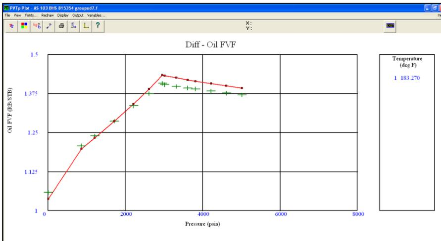
Figure. 12. Differential liberation test – Oil FVF match (RFR01 Oil sample)
