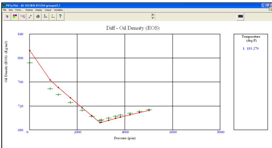
Figure. 13. Differential liberation test – Oil density match (RFR01 Oil sample)
