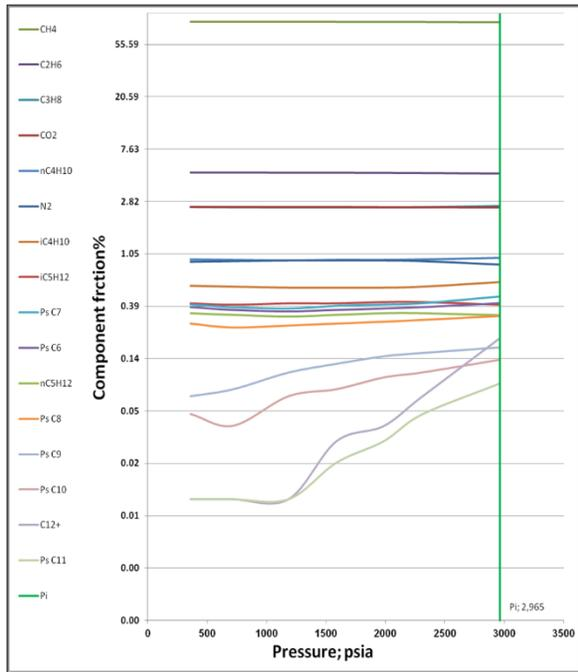
Figure. 2 Extending fluid components fraction from CVD to the initial pressure
