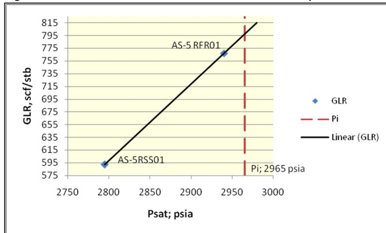
Figure. 15 Correction of Rsi for (RFR01 Oil sample)
