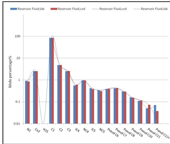
Figure. 5. Comparison between the original and the new stream fluid composition
