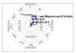
Fig. 4. Travelling cylinder plot of anti-collision well planning
