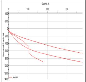
Fig.3 shows the clearance results between the subject well and offset well 1, offset well 2 and offset well 3. It shows from the graph that MD of these offset wells and their distance from the subject or planned wells. This graph summarizes the results obtained in table 1 to table 3 as shows that the three wells keep away from the planned well with adequate separation that maintains the separation control rule.
