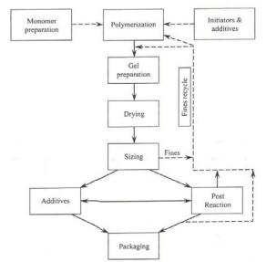
Figure 1. hydrogel preparation block diagram (solution polymerization procedure)
