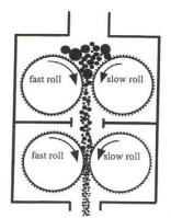
Figure 7. Schematic diagram of a two-pair high roll crusher
