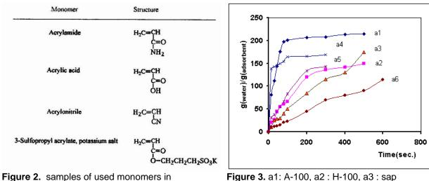
Figure 2. samples of used monomers in preparation of hydrogels.
