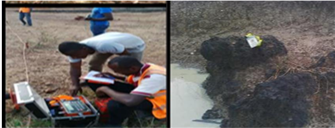
Figure 2. Pictures from the study area. (a) Data acquisition process at the study area, showing cable reel, electrode and resistivity meter (ABEM SAS 1000) (b) Rock formation in the study area
