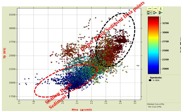
Figure 10. Cross plot of P-wave velocity against density (rho) with depth for Well X-004.
