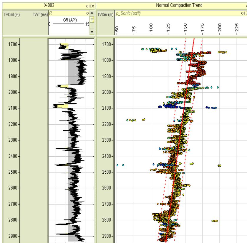
Figure 22. Normal Compaction trend on Compressional Sonic for X-002 Well indicating Onset of Overpressure and its Zones.
