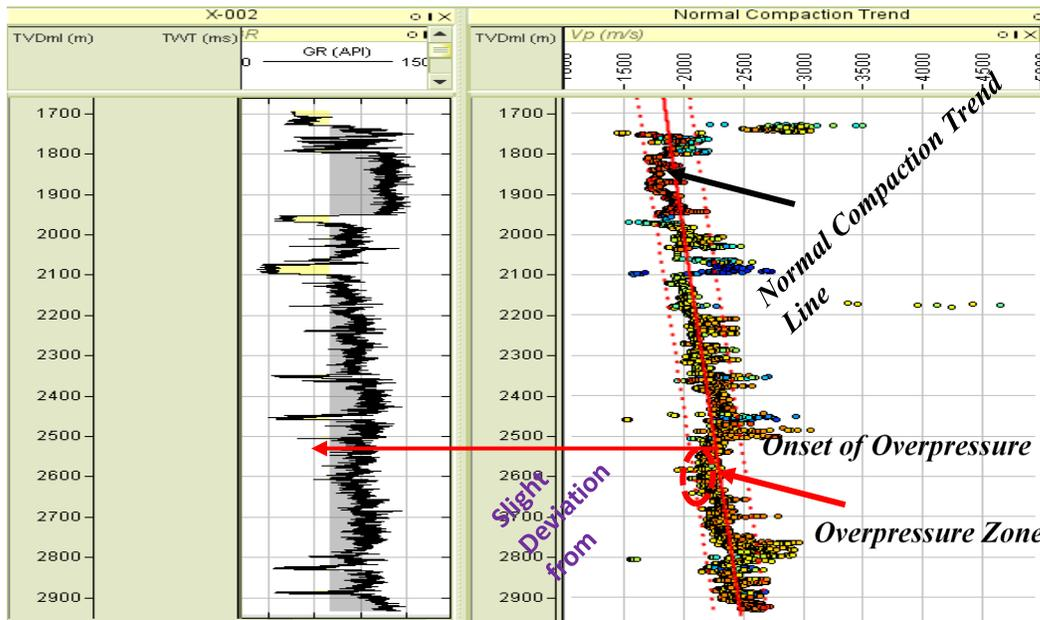
Figure 19. Normal Compaction trend on Compressional Velocity for Well X-002 indicating Onset of Overpressure and its Zones.
