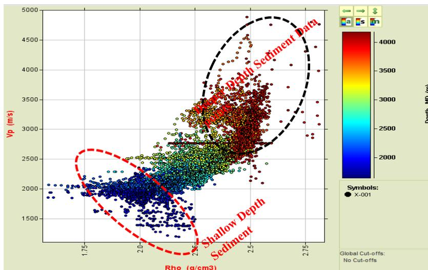
Figure 9. Cross plot of P-wave velocity ( $V_p$ ) against density ( $\rho$ ) with depth for Well X-001.
