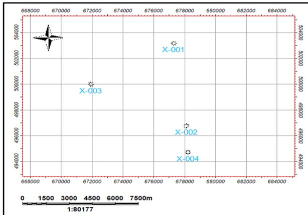
The base map (Figure 2) was generated after loading the available well log data with petrel™ 2014 software. The map depicts the distribution, orientation and location of the wells as well as the seismic grid lines. It is composed of drilled wells, direction of north and a linear scale.
