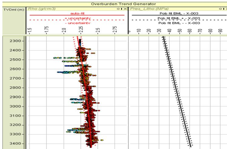
Figure 13. Overburden trend generated from the density log for Well X-003.
