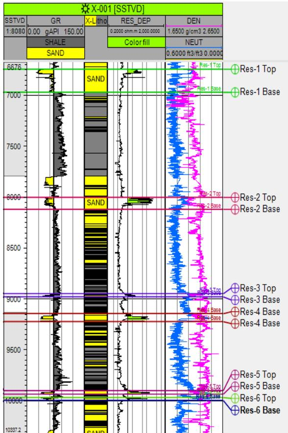
Figure 4. Lithological Delineation for Well X-001.
