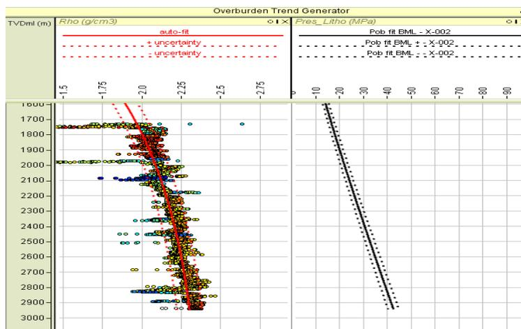
Figure 12. Overburden trend generated from the density log for Well X-002.
