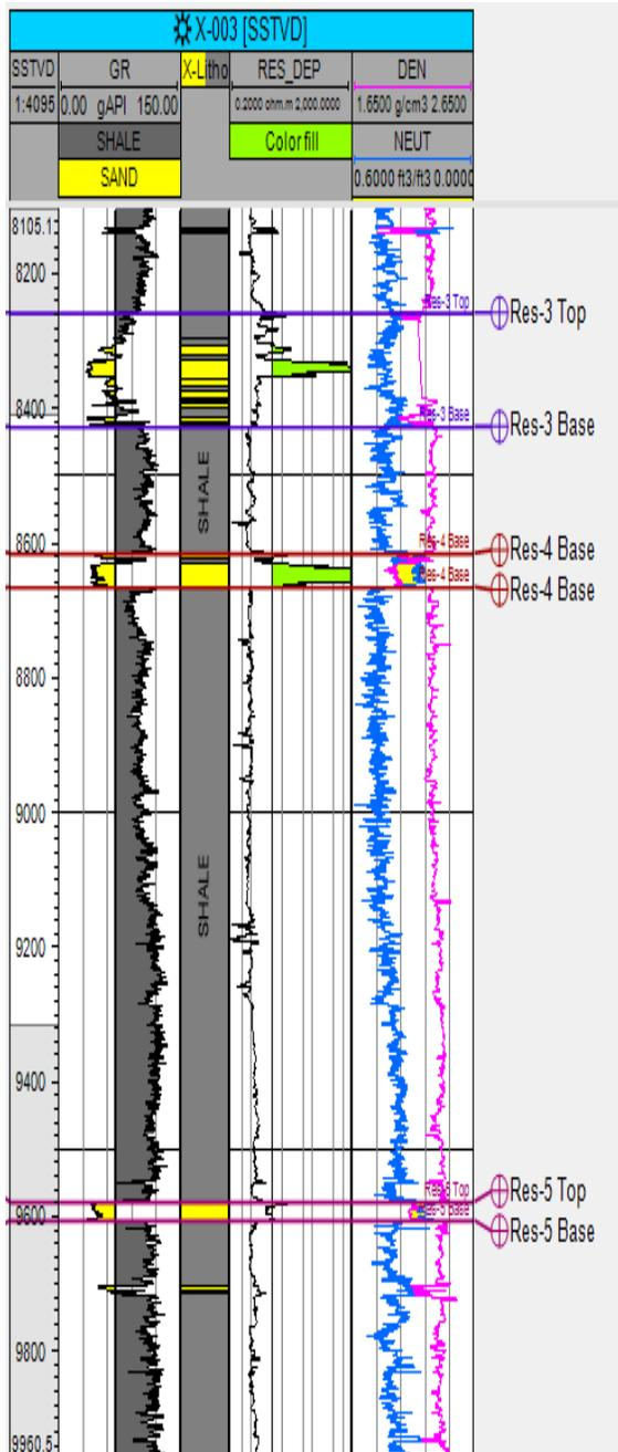
Figure 6. Lithological Delineation for Well X-003.
