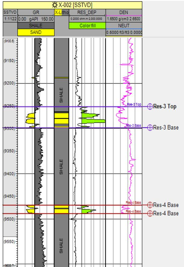
Figure 5. Lithological Delineation on Well X-002.
