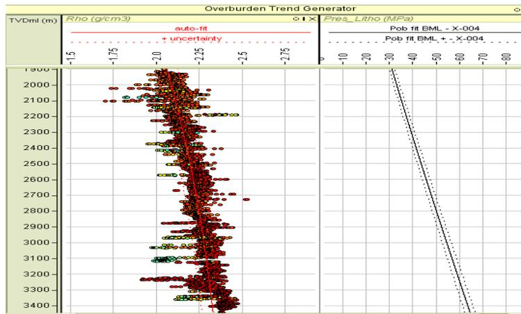
Figure 14. Overburden trend generated from the density log for Well X-004.
