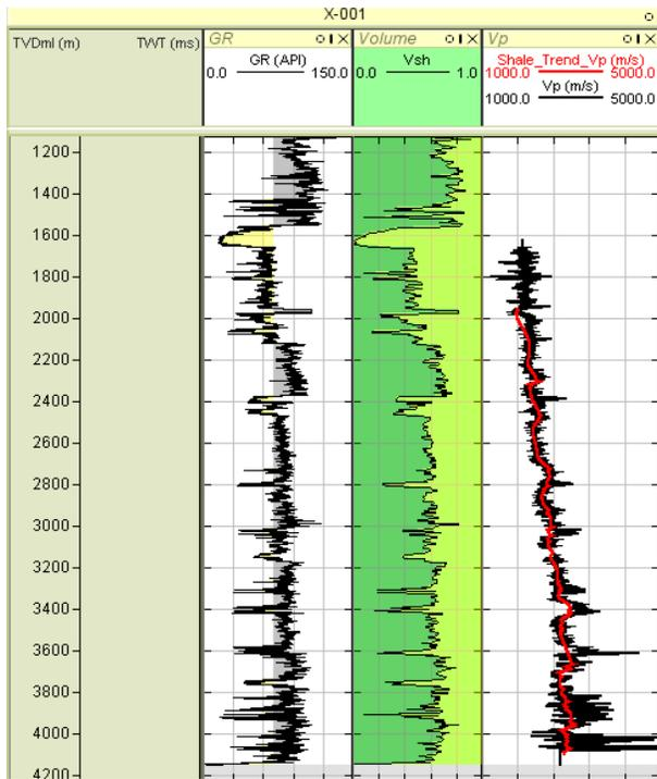
Figure 15. Display of Lithology and Compressional Velocity Shale trend for Well X-001.
