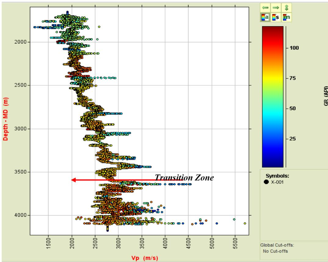
Figure 8. Cross plot of depth against P-wave velocity ( $V_p$ ) colour coded with GR for X-001 well.
