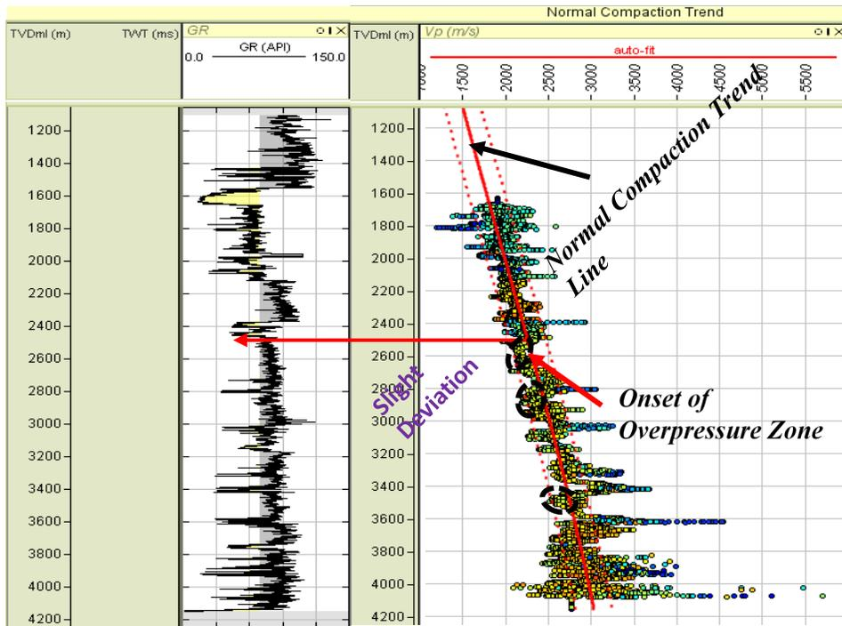
Figure 18. Normal Compaction trend on Compressional Velocity for Well X-001 indicating Onset of Overpressure and its Zones.
