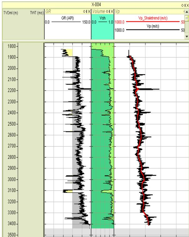
Figure 17. Display of Lithology and Compressional Velocity Shale trend for Well X-004.
