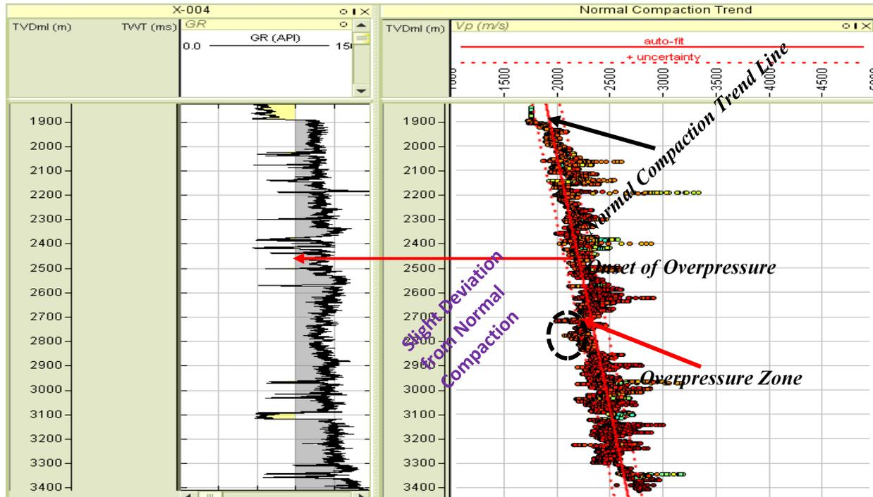
Figure 20. Normal Compaction trend on Compressional Velocity for Well X-004 indicating Onset of Overpressure and its Zones.
