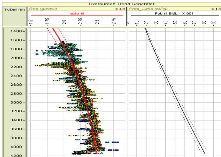
Figure 11. Overburden trend generated from the density log for Well X-001.
