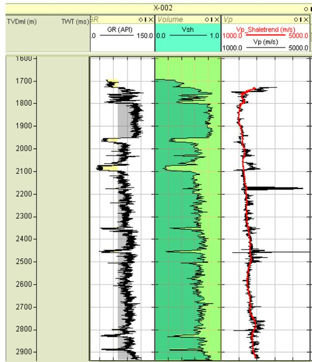
Figure 16. Display of Lithology and Compressional Velocity Shale trend for Well X-002.
