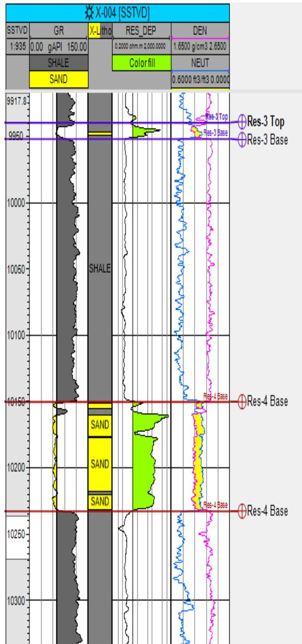
Figure 7. Lithological Delineation for Well X-004.
