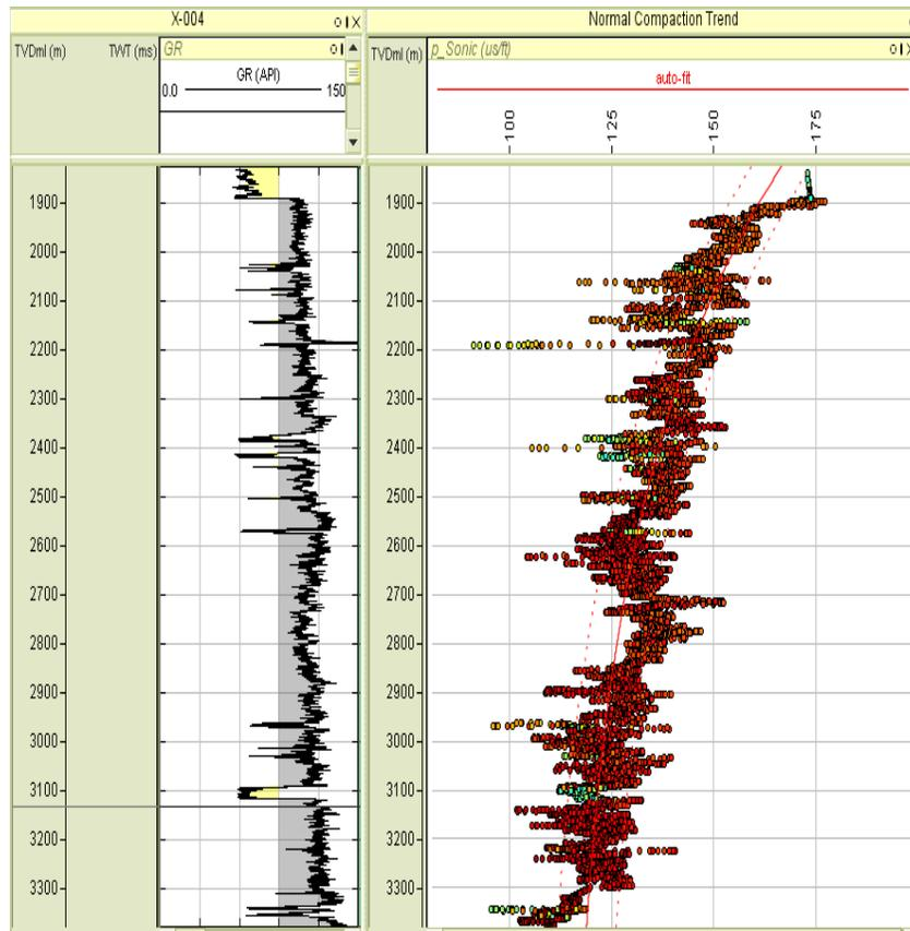
Figure 23. Normal Compaction trend on Compressional Sonic for X-004 Well indicating Onset of Overpressure and its Zones.
