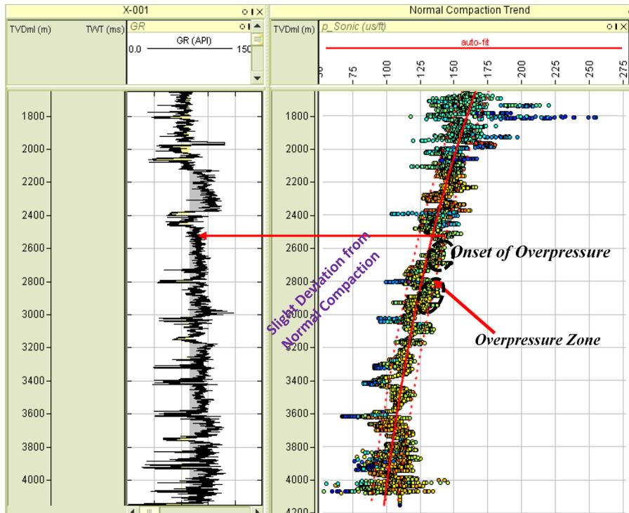
Figure 21. Normal Compaction trend on Compressional Sonic for X-001 Well indicating Onset of Overpressure and its Zones.
