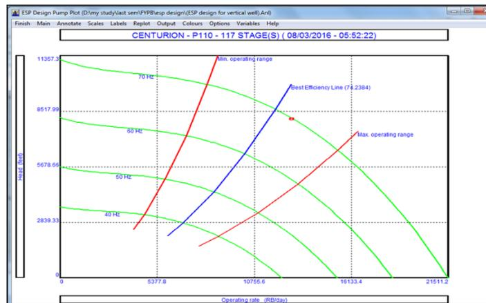
Fig 2. Pump efficiency curves for Centurion 562 P110 (vertical well-y)
