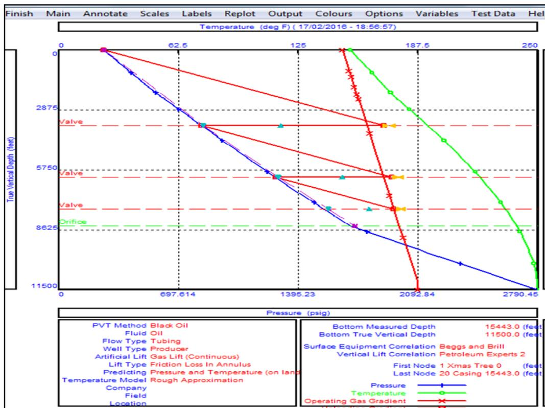
Fig. 7. Valves distribution for (horizontal well-x)
