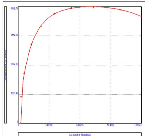
Fig 6. Gas lift performance curve for (horizontal well-x)
