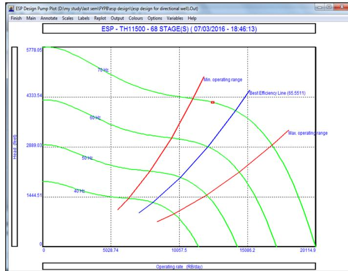
Fig. 4 Pump curves for ESP 562 TH11500 (horizontal well-x)
