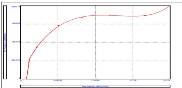
Fig. 5. Gas lift performance curve for (horizontal well-x)
