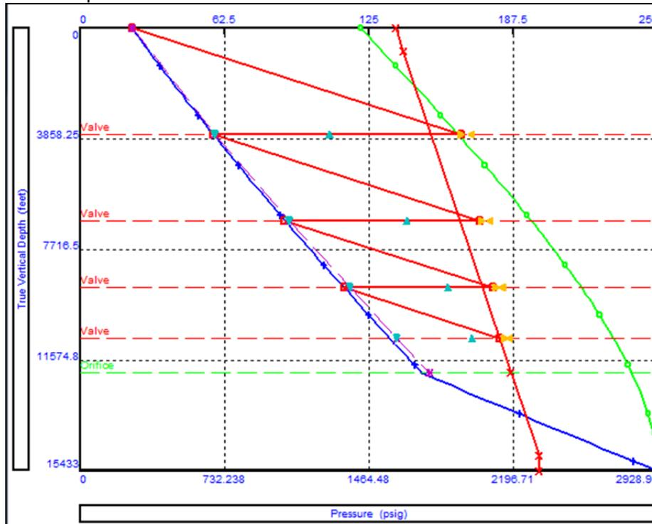
Fig. 8. Valves distribution for (vertical well-y)
