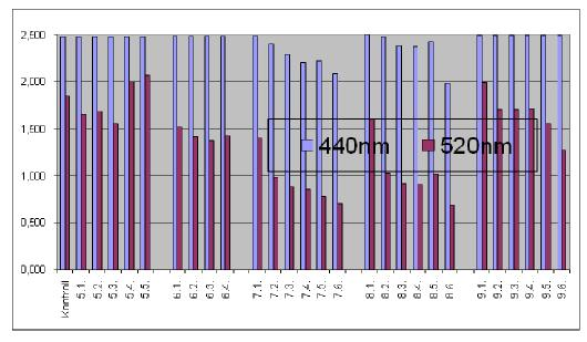
Figure 6. Adsorption treatment of refined ("kontroll") glycerine (series 5: fuller earth, series 6, 7, 8: ion exchange resins, Lanxsess, 9: activated carbon)
