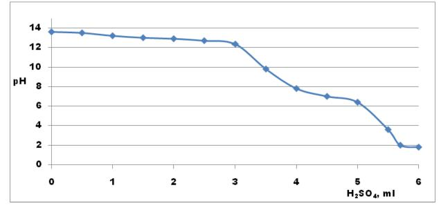
Figure 2. Titration curve of crude G-phase with concentrated sulfuric acid
