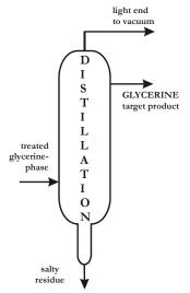
Figure 1. Standard industrial practice for producing glycerine by high vacuum distillation
