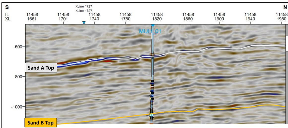
Fig. 9. An overlay of the generated synthetic seismogram on seismic inline 11458 showing a good tie with the seismic at the vicinity of MUH\_01 well.
