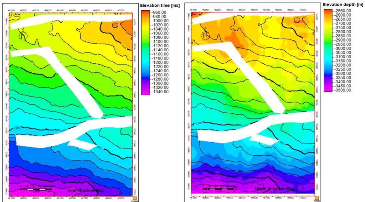
Fig. 13. Time and depth structure maps for Sand B reservoir top.
