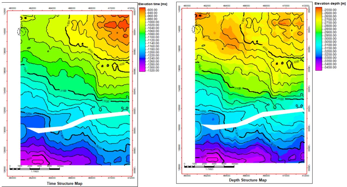
Fig. 12. Time and depth structure maps for Sand A reservoir top.
