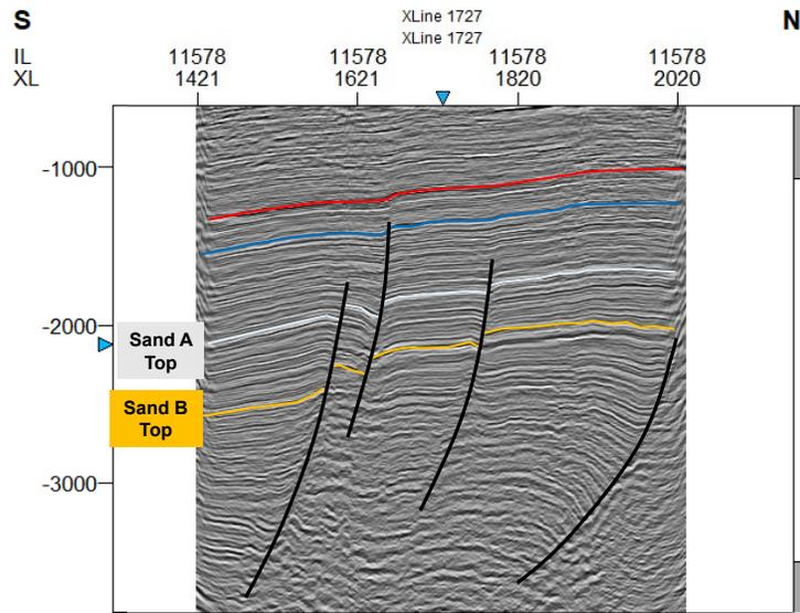
Fig. 10. Interpreted seismic section showing mapped horizons and faults in the study area.
