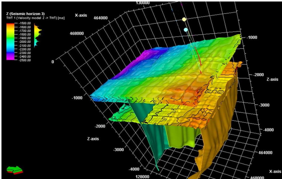
Fig. 14. Combination of fault framework model and interpreted horizons showing the structural disposition of the study area.
