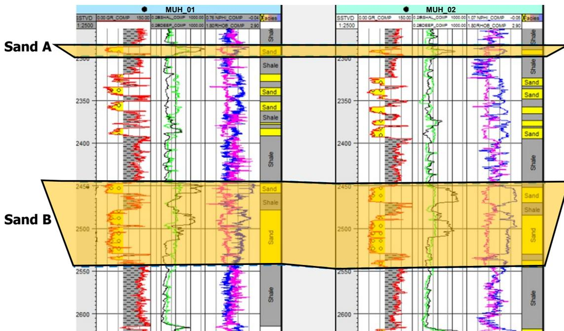
Fig. 7. Well log panel showing the delineated hydrocarbon-bearing sand units in the study area.
