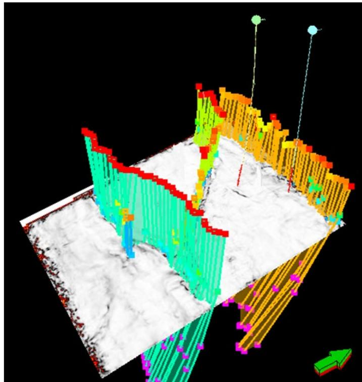
Fig. 11. 3D display of interpreted faults constrained by variance attributes time slice.
