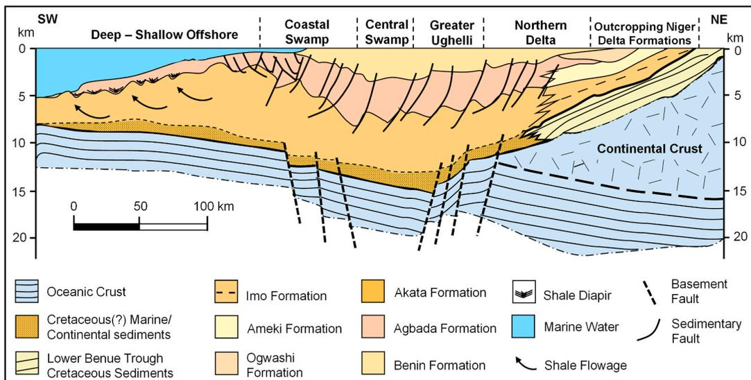
Fig. 3. Schematic diagram of the Cenozoic Niger Delta Basin showing the various depobelts, with the three diachronous lithostratigraphic formations and associated depositional structures (modified from [2,241]).
