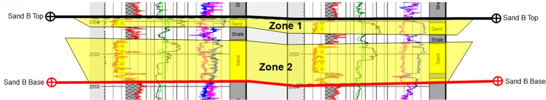
Fig. 8. Well log panel showing the two zones of Sand B reservoir.
