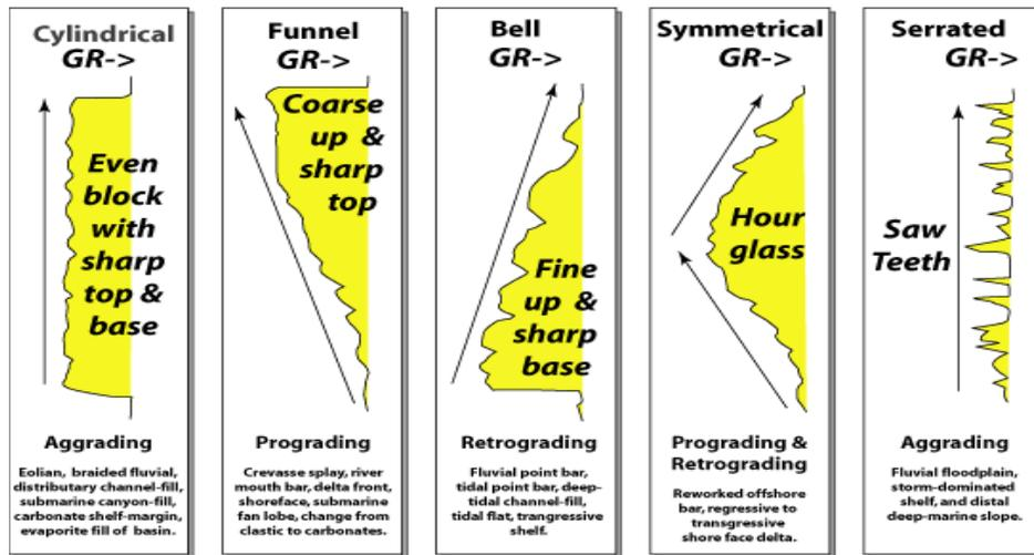
Fig. 4. Gamma ray response to grain size variation model (after [16]).
