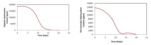
Fig. 3. Aliphatic hydrocarbon content biodegradation against time Fig. 4. Aromatic hydrocarbon content biodegradation against time
