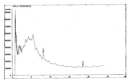
Fig. 1. GC-FID chromatogram showing the total aliphatic and aromatic hydrocarbon in crude oil before biodegradation
