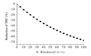
Fig.2 Reduction of total hydrocarbon (THC) emission by using biodiesel in diesel engine
