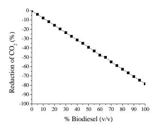
Fig.6 Reduction of CO<sub>2</sub> emission by using biodiesel in diesel engine
