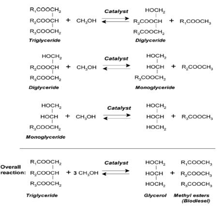
Fig. 1 Transesterification chemistry for methyl ester (biodiesel) production
