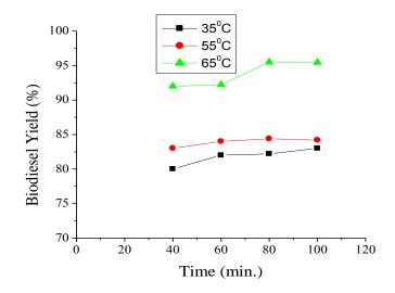
Fig. 3 Effect of temperature on transesterification
