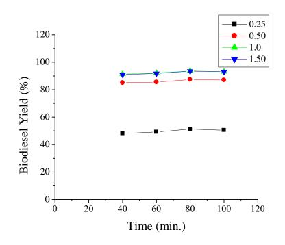
Fig.1 Effect of zinc oxide concentration on transesterification reaction
