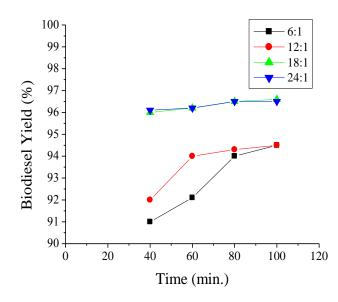
Fig. 2 Effect of ethanol-oil ratio on transesterification reaction
