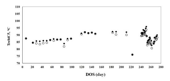
Figure 5. Comparison of the optimum (○) and actual (♦) temperature of de-isopentanizer reboiler vs. DOS
