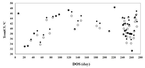
Figure 4. Comparison of the optimum (○) and actual (♦) de-isopentanizer condenser vs. DOS
