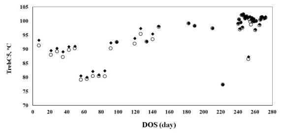
Figure 8. Comparison of the optimum ( $\circ$ ) and actual ( $\blacklozenge$ ) temperature of the de-pentanizer reboiler vs. DOS
