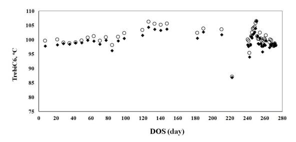
Figure 9. Comparison of the optimum (○) and actual (♦) temperature of de-isohexanizer reboiler vs. DOS
