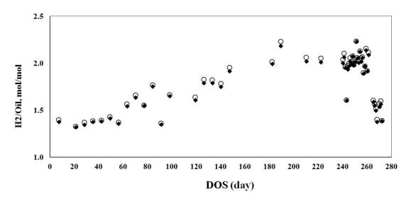
Figure 7. Comparison of the optimum (○) and actual (♦) hydrogen to hydrocarbon molar ratio vs. DOS
