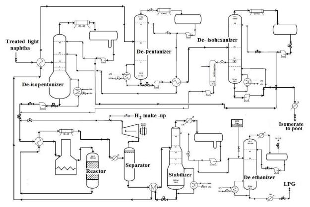
Figure 1. Block flow diagram of the light naphtha isomerization plant
