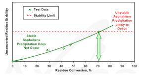
Fig.12 The stability limit for the ebullated bed hydro-cracking conversion level <sup>[10, 6]</sup>
