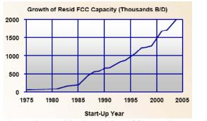
Fig.11 The worldwide residue FCC capacity growth <sup>[17]</sup>
