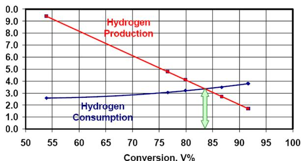
Fig. 13 Hydrogen Balance Point [6, 11]
