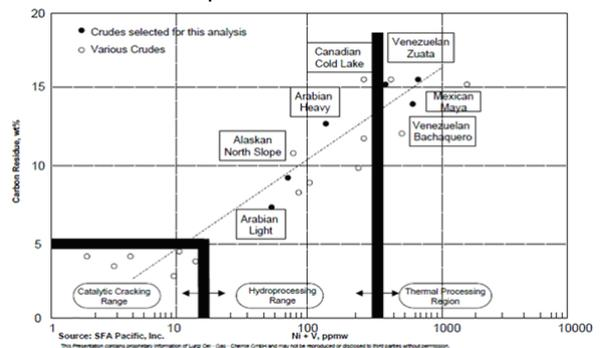
Fig. 6 Properties of 343°C+Boiling Point Residues [20]
