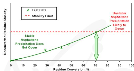
Fig.12 The stability limit for the ebullated bed hydro-cracking conversion level [10, 6]
